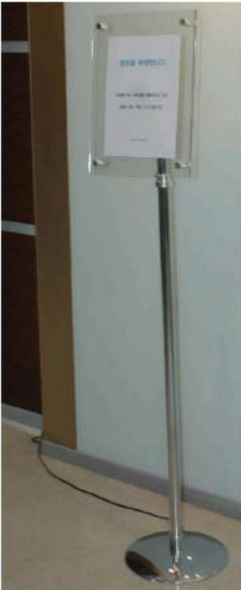
FILMSPEAKER is an ultra thin electrostatic speaker based on a PVDF film, which is both extremely spectacular and offers the possibility to apply any kind of visual display (paper, poster, picture etc..) so that you have a thin audio & visual communication tool.
