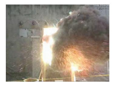
Bert Hickman's site, <u>Stoneridge Engineering</u> has a great page featuring high energy electrical failures and phenomenon. Along with video of an <u>exploding transformer substation</u> there's the <u>world's biggest jacob's ladder</u> and an awesome demonstration (pictured) of <u>high current</u>, <u>low voltage arcing</u>:
