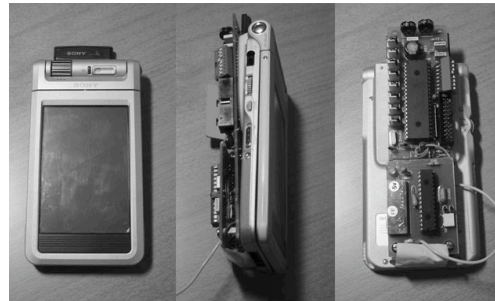
Figure 1. A PDA as mobile terminal with sensor subsystem
