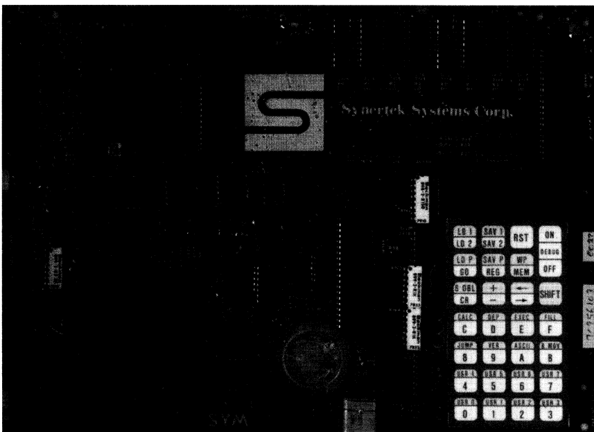
Fig. 1. In 1987 the hardware “hacking” environment of choice was the Synertek SYM 6502 single-board computer. Using Digital ADM3a terminals and a rudimentary assembler, Phil Stone wrote the software for Tim Perkis’s hardware configuration. The configuration allowed three users on each of the two SYMs to use the RS-232 serial protocol to communicate with a 1-K memory pad. This pad was shared by the two computer systems over the phone lines. In rehearsal, a null modem cable was used. (Photo: Scot Gresham-Lancaster)
